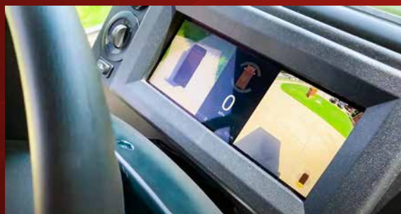
360° Camera System with Proximity Sensors
